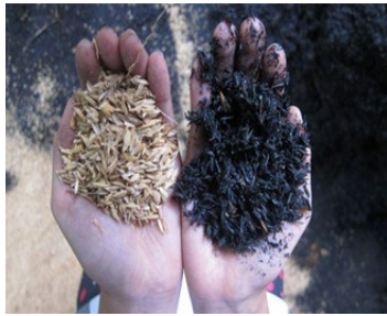
Completely burnt RH is grey to white in color, while partially burnt rice-husk ash is blackish
